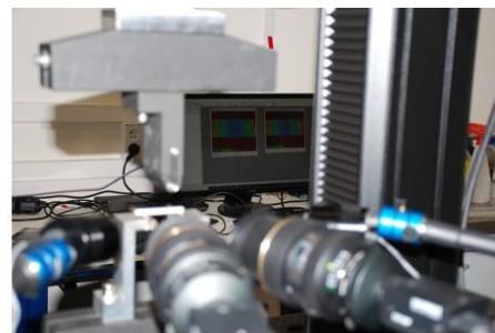
Three-point bending setup with DIC
